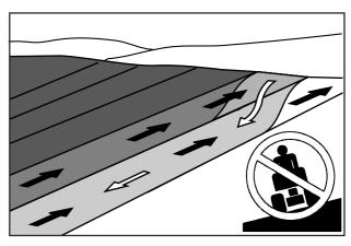
Cut slopes upwards and downwards, not sideways.
